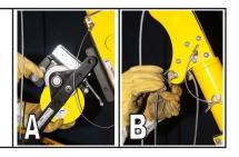
**WARNING:** It is strictly prohibited to use the material /positioning winch as a fall arrest, when the winch is positioned on the bottom mounting bracket located under the davit arm.
