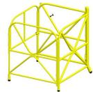
2. **A)** Undo the rubber draw latch and open the manhole guard to its maximum capacity. **B)** If necessary, adjust the legs to level the system. **C)** Close and lock the door using locking mechanism.
