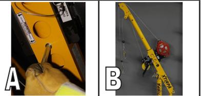
**IMPORTANT:** It is imperative to keep the pulling angle at a maximum of twenty-two degrees (22°) from the lifeline cable or rope, as to avoid any frontward load unbalance of the manhole guard and cause it to topple over (see illustration A).
