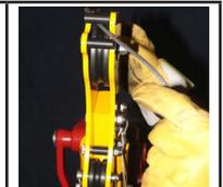
8. **A)** If a material positioning winch is required, use the bottom mounting bracket located under the davit arm. Install winch to mounting bracket and lock with pin attached to winch. **B)** Remove the small pulley locking pin. Position cable over pulley and re-install pulley using locking pin.
