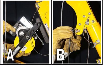
**WARNING:** It is strictly prohibited to use the material /positioning winch as a fall arrest, when the winch is positioned on the bottom mounting bracket located under the davit arm.
