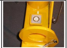
**WARNING:** Make sure that the system is well-positioned and that all components are locked into place with the pin provided for that purpose.
