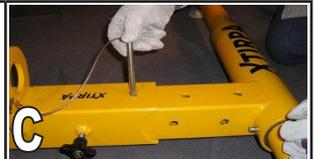
**IMPORTANT:** Make sure that all pins are locked in tightly.
