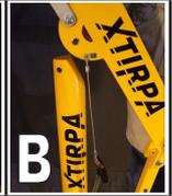
8. A) Lock everything with the first handle pin. B) Install the inferior leg of the davit arm between the eyelets of the mast and lock with the second handle pin.
