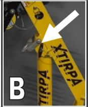
10. Pass the lifeline cable or rope through the pulley located at the top end of the davit arm. Make sure that the lifeline cable or rope is well in place.
