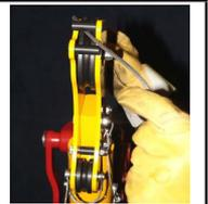
11. A) If a material positioning winch is required, use the bottom mounting bracket located under the davit arm. Install winch to mounting bracket and lock with pin attached to winch. B) Remove the small pulley locking pin. Position cable over pulley and re-install pulley using locking pin.
