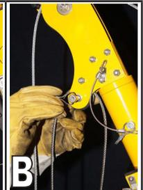
**WARNING:** It is strictly prohibited to use the lifeline cable / positioning winch as a fall arrest, when the winch is positioned on the bottom mounting bracket located under the davit arm.
