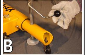
**WARNING: B)** After adjusting the base to the desired width, the system must be raised so that the wheels are not touching the ground. Only the adjustable support legs should support the base.
