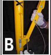
9. A) Install the lifeline or winch onto the gallow's bracket designed to accept this type of equipment. Use the locking pin provided with the lifeline or winch bracket and lock with the pin. B) A second lifeline can be installed on the grey "D" anchor point.
