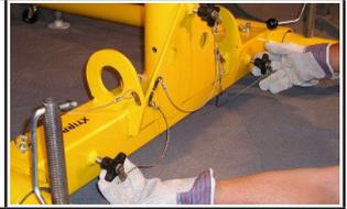
5. When the base is in position, make sure to use the adjustable support legs to make the system level. Use a level and make sure that the bubble is in the center of the indicator.
