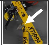
7. Remove the retaining pin located at top of davit arm. Pass the lifeline cable or rope into the pulley located at the top end of the davit arm. Be assured that the lifeline cable or rope is well in place.
