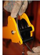
8. Safely replace the retaining pin.
