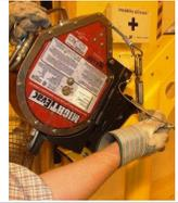
5. A second lifeline or winch can be installed on the jib. Install the lifeline or additional winch on the support of the jib designed to receive this type of equipment. Use the locking pin supplied with the lifeline or winch support and lock everything with the latter.
