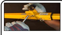
4. A. Remove the pulley from the center of the pole, cross the cable under the pulley and put back the pulley in position and secure by using the locking pin.
