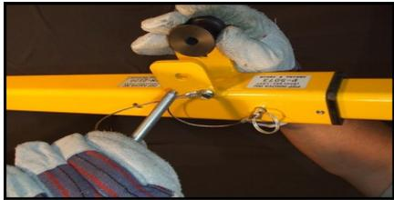
4. **A.** Remove the pulley from the center of the pole, cross the cable under the pulley and put back the pulley in position and secure by using the locking pin.
