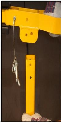
1. Make sure that all the components and the parts are in perfect working order and that everything works correctly. Remove the pins of the pole hoist, install the T-bar and secure everything with the locking pin.
