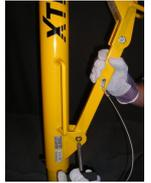
**WARNING:** Make sure that the system is in the right position and that all components are locked with the provided pin.
