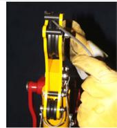
4. If a material / positioning winch is required, use the bottom mounting bracket located under the davit arm. Install winch to mounting bracket and lock with pin attached to winch.
