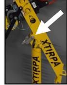
3. Install the lifeline cable or rope or winch on mounting bracket made to accept the hoisting device. Pass the lifeline cable or rope into the pulley located at the top end of the davit arm. Make sure that the cable or rope is securely in place.
