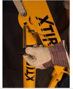
11. Install the lower leg of the davit arm between the eyelets of the mast and lock it with the second pin.
