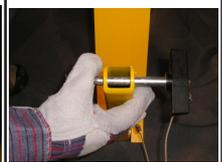
9. Install the receptacle of the davit arm on the mast.
