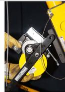
5. Remove the small pulley locking pin. Position cable over pulley and re-install pulley using locking pin.
