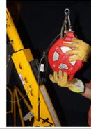
2. A second lifeline can be installed on the gray "D" anchor point.
