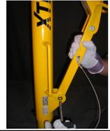
**WARNING:** Make sure that the system is in the right position and that all components are locked with the provided pin.
