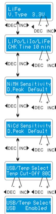
The screen shows the nominal voltage of Lithium battery. There are three kinds of Lithium battery: LiFe(3.3V),LiIo(3.6V) or LiPo(3.7V). This information is of critical importance that you have to check the battery carefully to make sure it is set up correctly. If it is different from correct value, explosion can occur during charge process.
