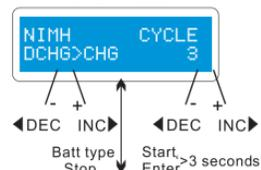
You can set up sequence on the left and the number of cycles on the right. You can balance, refresh and break-in the battery with this function. You can set a temporary cool-off procedure in the user's setting. Range of the cycle number is 1-5.
