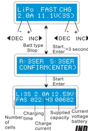
The value on the left side of the second lines sets the charge current. The value on the right side of the second lines sets the battery pack's voltage. After setting current and voltage, press START/ENTER for more than 3 seconds to start the process.
