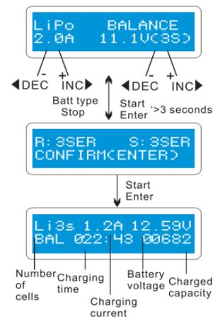
The left side of the first line shows the type of battery you choose. The value on the left of the second line of the charger is current user set. After setting the current and voltage, press START/ENTER key for more than 3 seconds to start the process. (charge current: .1-5.0A, voltage: 1-5V).
