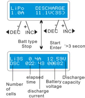
The value of discharge current on the left cannot exceed 1C, and the value on the right cannot be under the voltage recommended by the manufacturer to avoid deep discharging. Press STAR/ENTER for more than 3 seconds to start charging.
