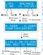
The left side of the first line shows the type of battery you choose. The value on the left of the second line of the charger is current user set. After setting the current and voltage, press START/ENTER key for more than 3 seconds to start the process. (charge current: .1-5.0A, voltage: 1-5V).
