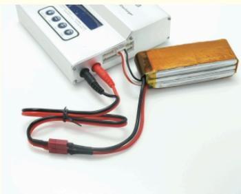
\*The main battery leads must be connected along with the balance lead connector as shown before charging your battery.
