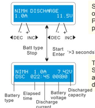
The screen indicates the discharging state. You can press START/ENTER key to alter discharge current. Press START/ENTER again to store the value. Press BATT TYPE/STOP key to stop discharging. The emitted sound alerts the end of discharging.
