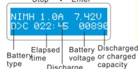
Press BATT TYPE/STOP key to stop program, you can press START/ENTER key to alter charge current. The sound indicates the end of program.
