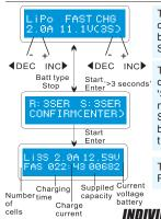
The value on the left side of the second lines sets the charge current. The value on the right side of the second lines sets the battery pack's voltage. After setting current and voltage, press START/ENTER for more than 3 seconds to start the process.
