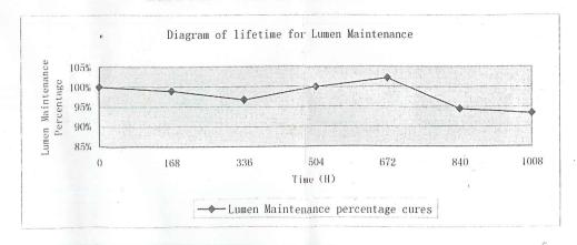
Testing Module:Lasting 1000 hrs, Temperature Range 36-40°C, Humidity:60%RH, Input Voltage:DC12V
