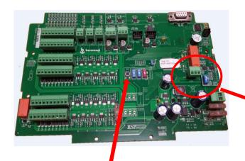
To pair the remote controls on the "EXTENDED" version board, we must first unlock the memory module.
