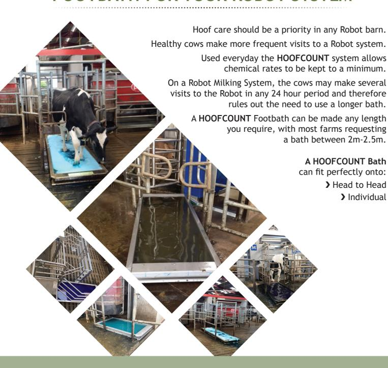
At 3.6m long and made slightly deeper than the Standard Hoofcount Bath, the **EXCEL BATH** allows 3 dips per hoof each time the cow passes through the bath.
