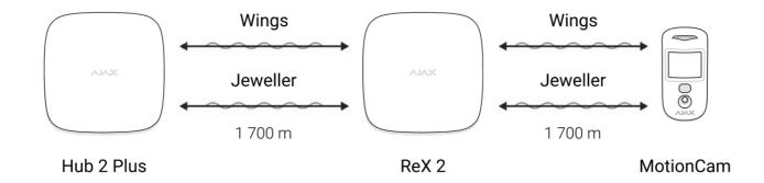
The communication range between ReX 2 and the device is limited by the radio signal range of the device. Radio signal range is indicated on the device page **on the website** and in the User Manual.
