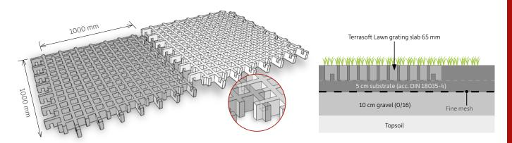
The Terrasoft Lawn Grating Slabs interlock with one another in a form-fitting manner. Laying in half-staggered offset formation offer a sustained connection.
