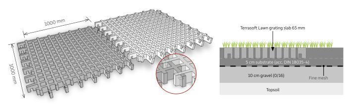
The Terrasoft Lawn Grating Slabs interlock with one another in a form-fitting manner. Laying in half-staggered offset formation offer a sustained connection.
