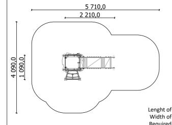
Lenght: Width: 2 210 mm 1 090 mm Height: 2 380 mm Lenght of safety area: 5 710 mm 4 090 mm Width of safety area: 18 m<sup>2</sup> Required safety area: (Install shock absorbing material according to EN 1176:2017)
