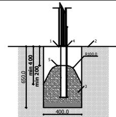
Playground equipment steel foundation is concreted in the ground at the planned location. The equipment can be used after two days when the concrete becomes solid. During assembly no children are allowed in the area.
