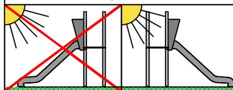
Foundation should be accessible for maintenance.
