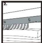
2. Use one finger and press / bend so that the free sheet metal fingers fill in the spaces towards the lid boards.
