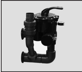
2) MULTI-POR-T VALVE + FITTINGS 20" model supplied with 1½" MPV. 24", 30" and 36" models supplied with 2" MPV.
