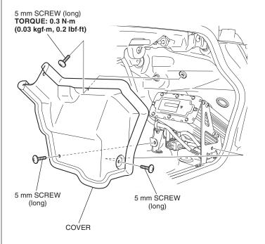
92. Install the 5 mm screw as shown.
