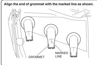
68. Install the hole plug as shown.
