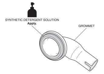
67. Install the grommets as shown.
