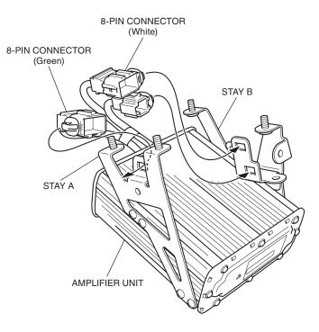
72. Install the amplifier unit as shown.
