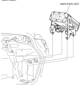
73. Install the 5 mm nuts as shown.
