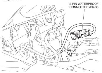
27. Remove the clip and disconnect the connector as shown.
