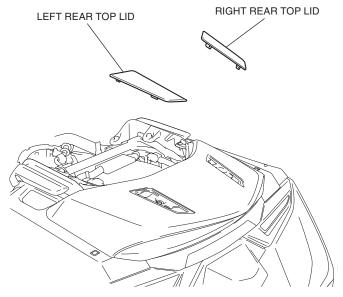
11. Remove the parts as shown.
