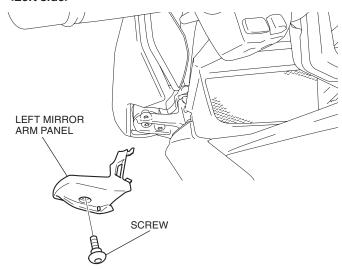
16. Remove the left rear view mirror as shown.
