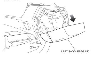
5. Remove the left side cover as shown, and disconnect the negative (-) cable of the battery.
