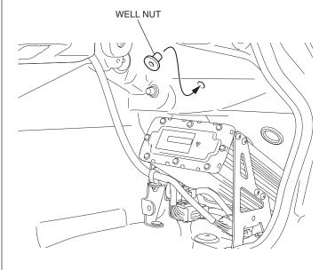
89. Clean the surface of the area shown using an isopropyl alcohol.
