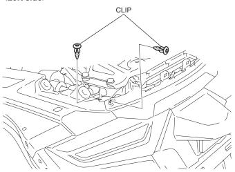
37. Remove the rear fender as shown.
