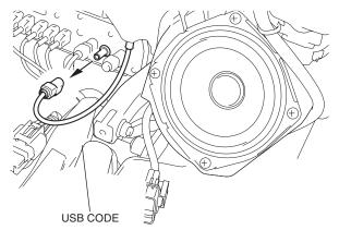
14. Disconnect the connector as shown.
