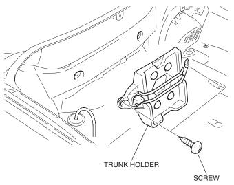
9. Remove the front trunk lower panel as shown.
