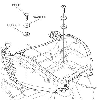
20. Remove the rear trunk as shown.
