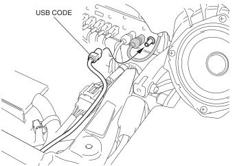
33. Secure the USB code with the wire tie as shown.
