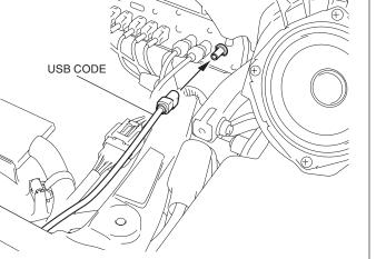
32. Secure the USB code with the wire tie as shown.
