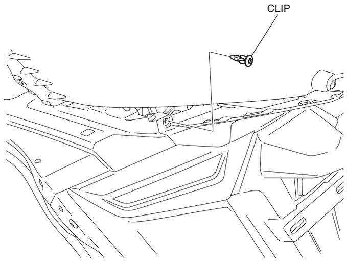
19. Remove the rear fender as shown.
