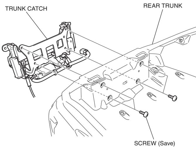
17. Remove the emergency trunk cable to the trunk catch as shown.
