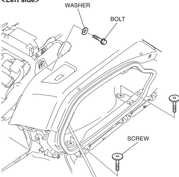
22. Remove the screw as shown.
