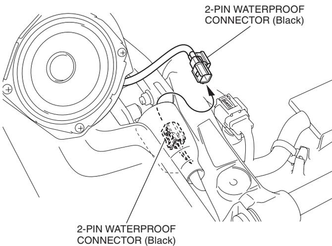
37. Install the dummy connector as shown.
