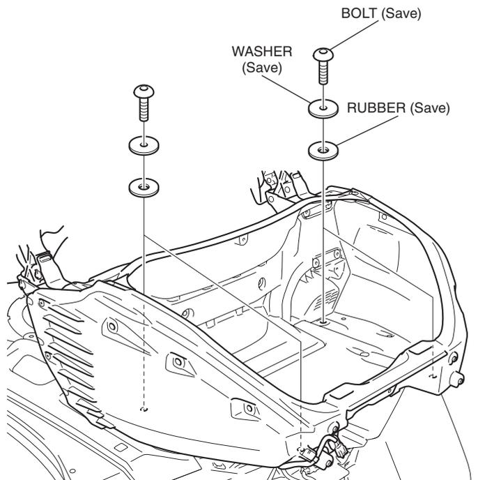
39. Remove the rear trunk as shown.
