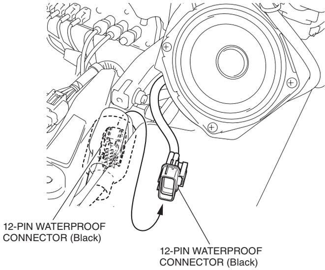
35. Install the dummy connector as shown.
