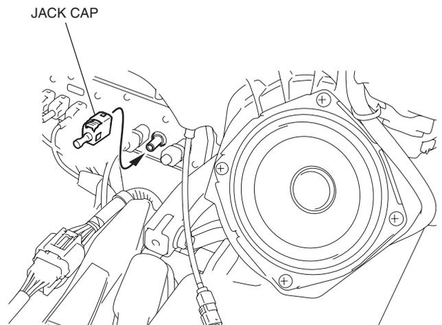
34. Disconnect the connector as shown.
