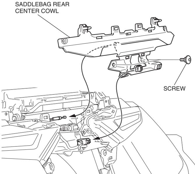
21. Remove the parts as shown.
