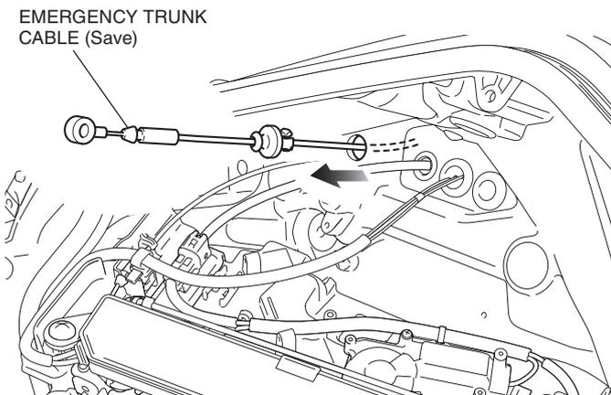
29. Apply synthetic detergent solution to the position shown.
