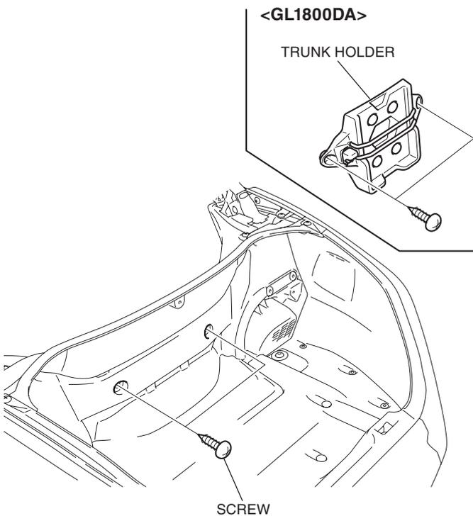
11. Remove the front trunk lower panel as shown.
