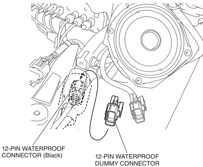
36. Disconnect the connector as shown.
