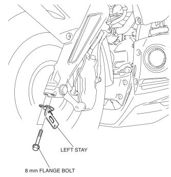
3. Install the left front caliper cover as shown.
