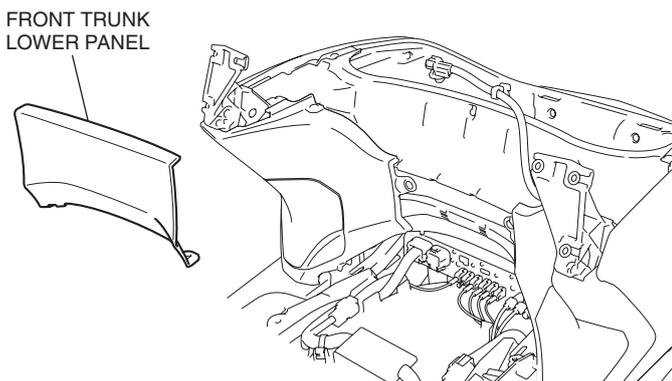
14. Remove the parts as shown.
