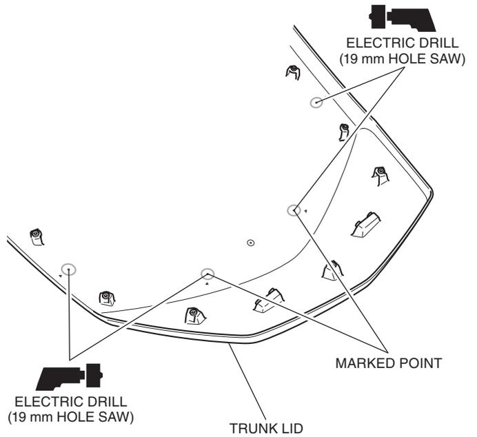
32. Install the grommets as shown.
