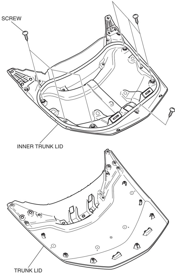
30. Drill at the marked points of the inner trunk lid as shown.
