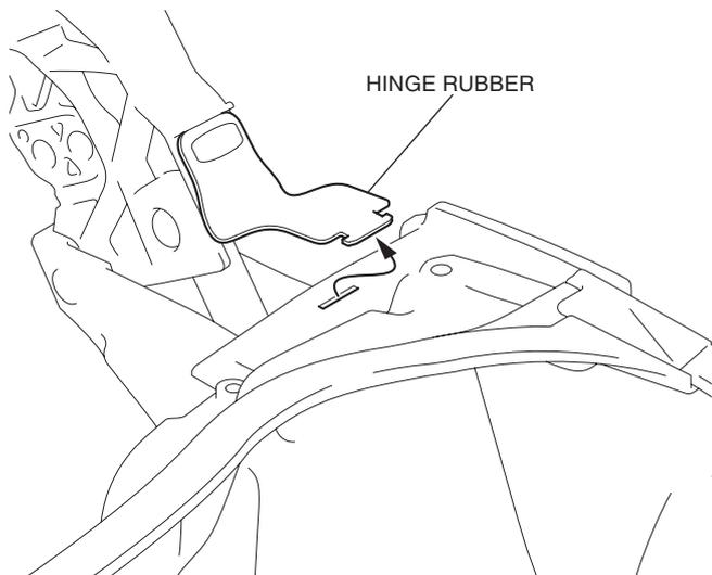
18. Remove the right trunk hinge as shown.
