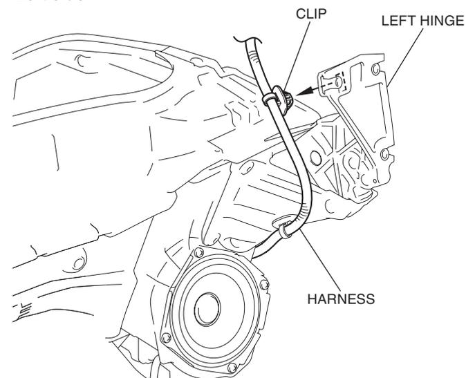
17. Remove the hinge rubber as shown.
