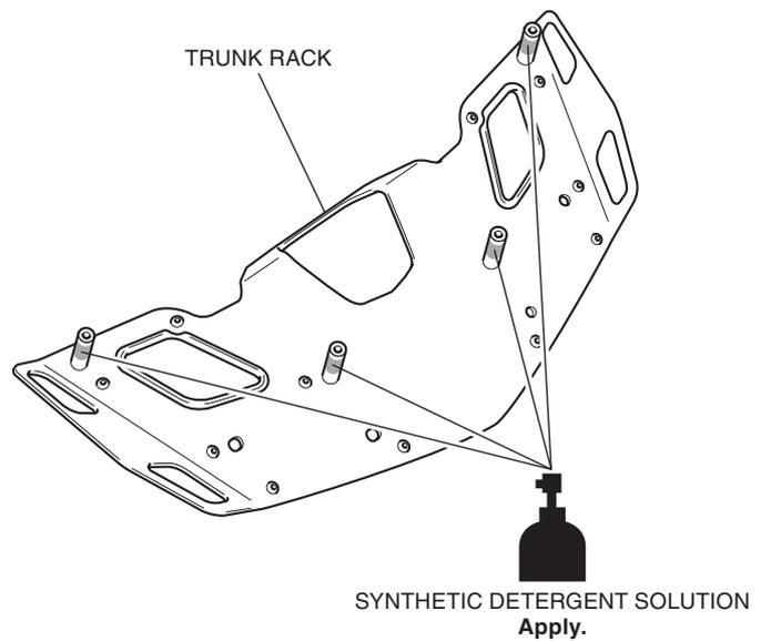
43. Install the trunk rack as shown.
