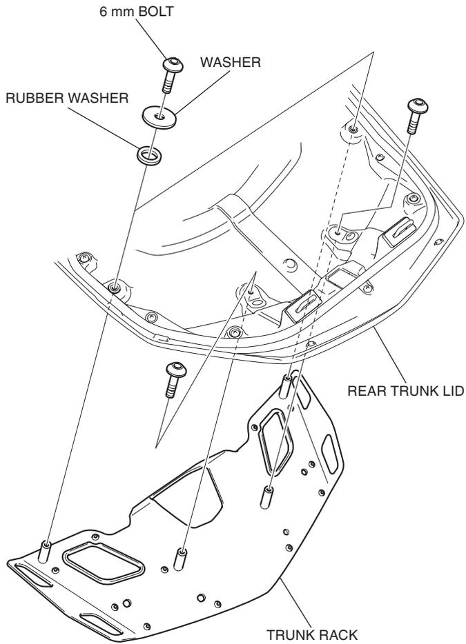
44. Install the rear trunk lid in the reverse order of removal.
