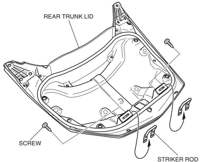
29. Remove the inner trunk lid as shown.
