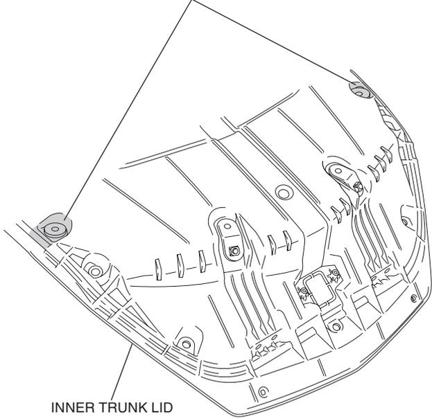
38. Attach the masking tape as shown.
