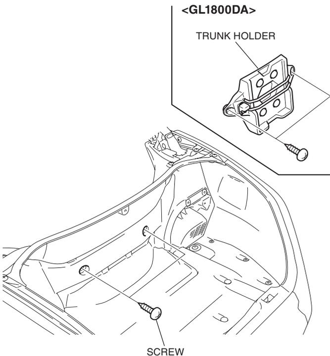
13. Remove the front trunk lower panel as shown.
