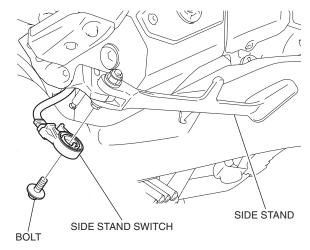
3. Remove the pivot bolt and side stand as shown.
