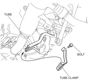
5. Apply synthetic detergent solution to the position shown.
