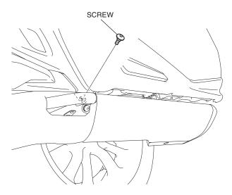
3. Remove the left exhaust pipe cover as shown.
