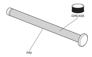
7. Pass the pin through the backrest bracket and arm.
