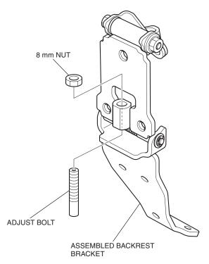
10. Install the special nuts as shown.
