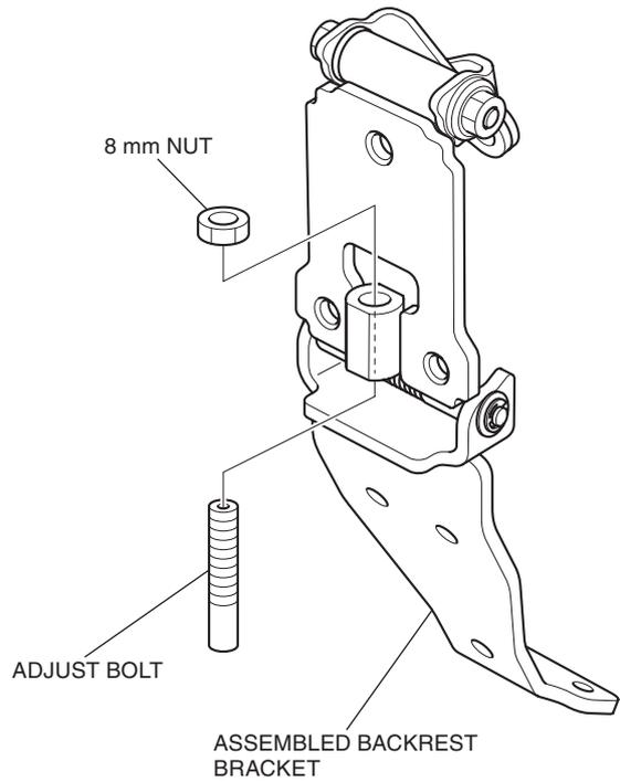
10. Install the special nuts as shown.
