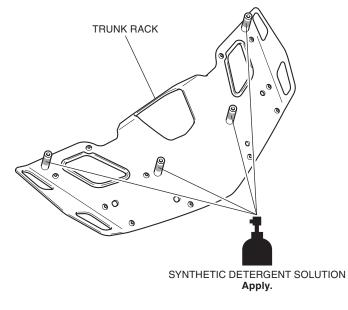
36. Install the trunk rack as shown.
