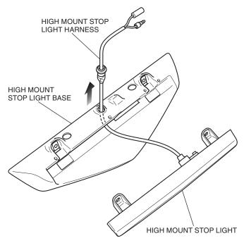
27. Install the high mount stop light as shown.
