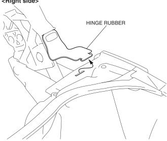
4. Remove the right trunk hinge as shown.
