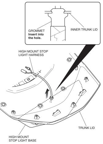
29. Clean the surface of the area shown using an isopropyl alcohol.
