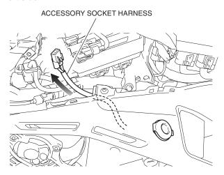
29. Remove the dummy connector as shown.
