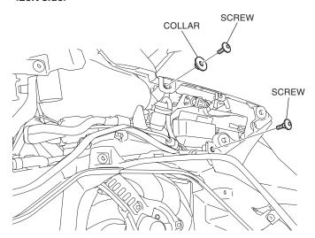
17. Remove the connector as shown.
