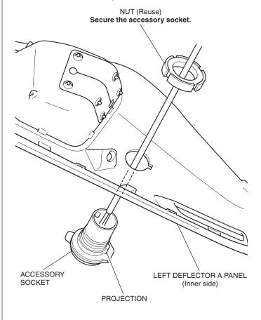
28. Route the accessory socket harness as shown, and install the left deflector A panel and parking lever in the reverse order of removal.
