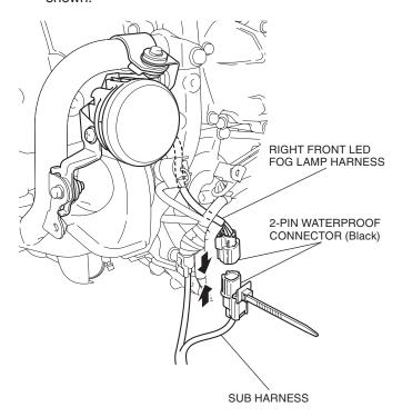
60. Secure the right front LED fog lamp harness with the wire tie as shown.
