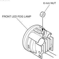
42. Loosely install the fog lamp adjust as shown. **<Left side>**
