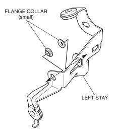
45. Loosely install the assembled left stay to the assembled front LED fog lamp as shown.
