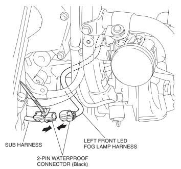
64. Secure the left front LED fog lamp harness with the wire ties as shown.
