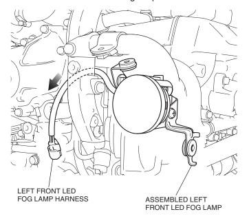
52. Install the assembled left front LED fog lamp as shown
