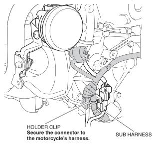
62. Route and secure the sub harness with the wire tie as shown.
