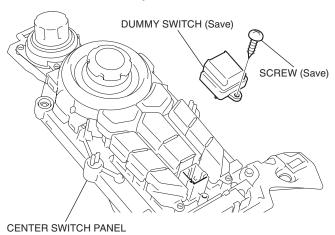
36. Install the fog lamp switch as shown.
