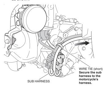
63. Connect the left front LED fog lamp harness as shown.
