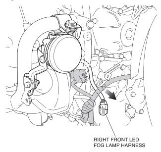
56. Remove the dummy connector as shown.
