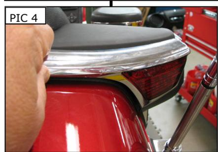
**STEP 7** Rub the backing paper of the Accent with your fingernail to activate the adhesive. Remove the backing paper and attach the Accent to the back of the passenger armrest. Press in place for one minute, full bonding will occur in 24 hours. Repeat Steps 4 and 5 for the left side.
