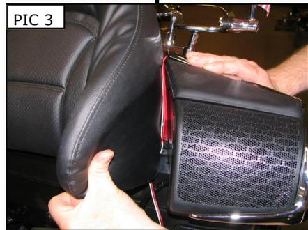
**STEP 6** Test fit the right Armrest Accent to the rear of the right passenger armrest. PIC 4 The Accent should follow the contour of the trunk and line up with the top of the passenger armrest. Make any reference marks along the outside edges of the Armrest Accent with a non-permanent marker or masking tape.
