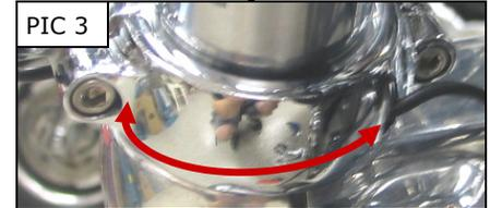
**STEP 8** Turn the handlebars lock to lock to make sure there is clearance between the lights and any component on the motorcycle.
