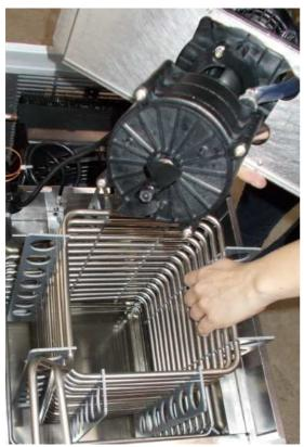
• Place the cooling coil into the water tank
