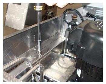
• Screw the holder of the pump in place again (on both sides)
