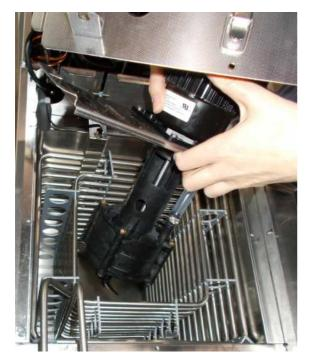
• Place the pump into the water tank again
