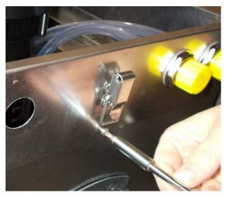
Remove the Torx screw of the connection plate
