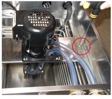
Remove the Torx screws of the pump holder (on both sides)
