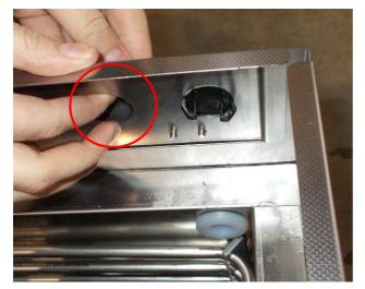
• Remove the blind cap of the connection plate
