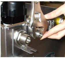
Screw also the new connections with the washers and the nuts together
