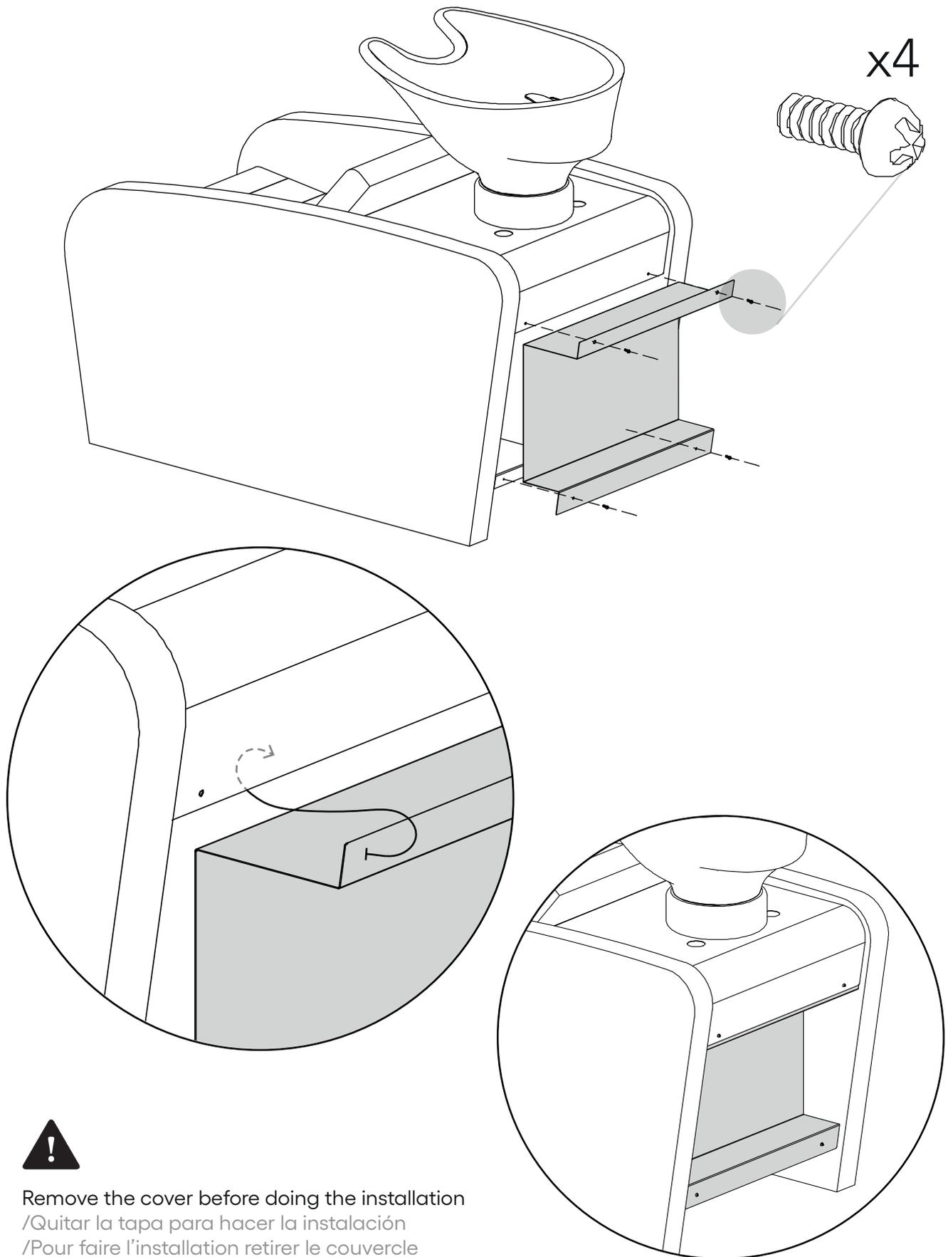
Remove the cover before doing the installation
