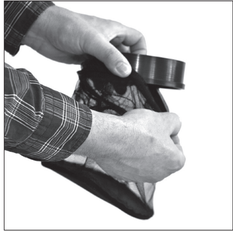
Attach net to quick lock adapter.
