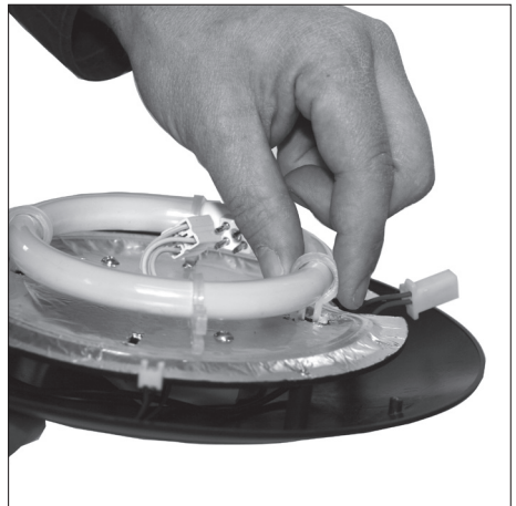
Disconnect 4 x tube holders (finch and turn gently inwards). Snap off the tube holders and attach them to the new tube.
