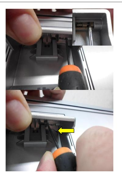
Insert the screwdriver into the hinge slot
