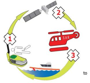
The 406 MHz frequency is a worldwide dedicated emergency frequency that is detected by a network of satellites called the Cospas-Sarsat system. This satellite system was established by,
