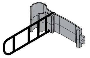
Attaching Oral Inflation Clip (with Mounting Strap Attached) to Beacon
