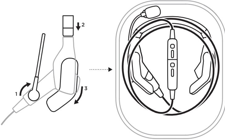
1. Rotate the microphone up to the headband.
