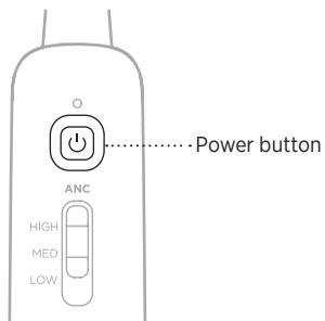
The Power light glows amber then blinks according to the power level.
