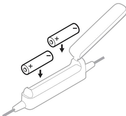
**CAUTION:** If the batteries don't fit correctly, do NOT force them in. Forcing an improper connection will cause permanent damage to the control module.
