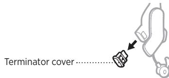
5. On the left side, align the release button to the release button opening, and insert the terminator cover into the base of the connector socket.
