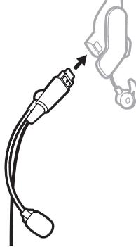
8. Slide the microphone connector into the connector socket until the release button is secure.
