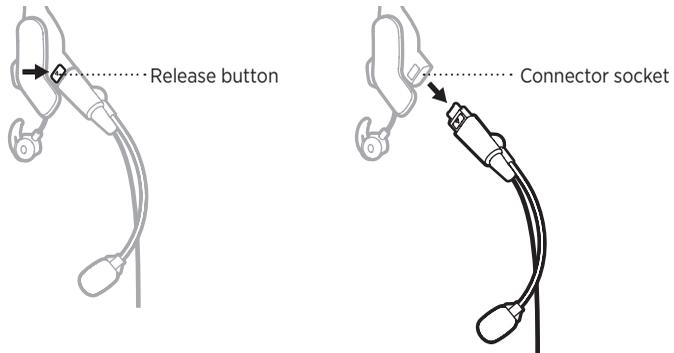
4. On the right side, push the release button, and gently pull the terminator cover from the connector socket.
