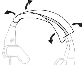
2. Place the new headband cushion under the headband with adhesive facing rear.
