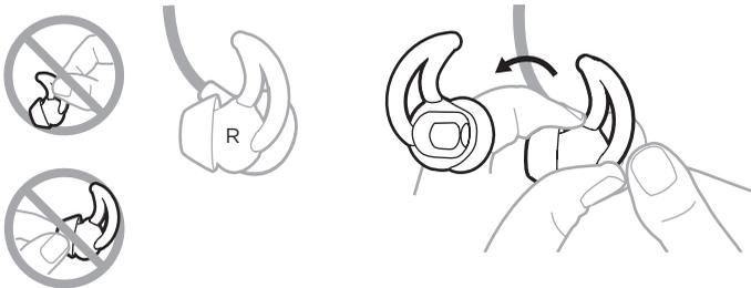
2. Align the opening of the new StayHear+ tip with the earbud nozzle and rotate the tip onto the nozzle. Press the base of the tip until it clicks securely into place.
