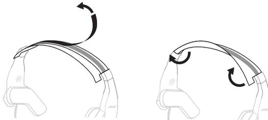
5. Insert the left and right tabs into the plastic cap.
