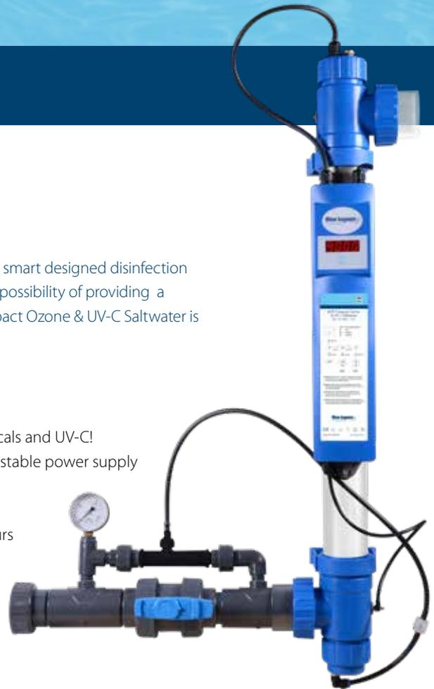
The 185nm radiation converts the available oxygen into ozone. The produced ozone (max. 0,6 g/h) is mixed with water through the venturi to perform its disinfecting/oxidising job. Inside the UV-C housing, any residual ozone will be converted by the 254nm UV-C radiation into OH radicals (the so called Advanced Oxidation Process) that have an even stronger oxidising power than ozone.
