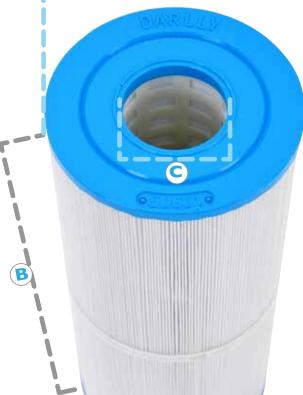
Measure the inside diameter of the opening of the cartridge or the inside edges of the thread. Holes are normally 50mm (2"), 75mm (3") or 100mm (4") Threads are normally 38mm (1 1/2") or 50mm (2")
