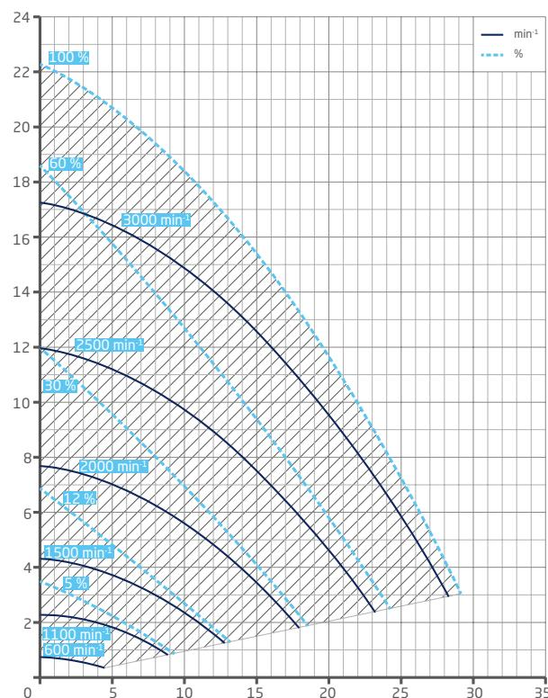
Total dynamic head  $H$  ( $\text{m}$ ) / Flow rate  $Q$  ( $\text{m}^3/\text{h}$ ) >
