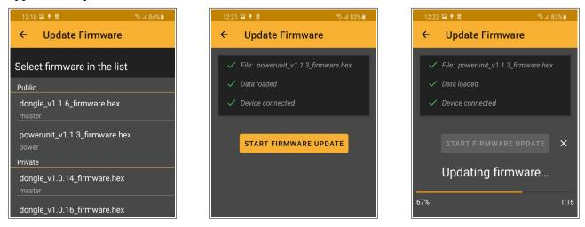
**Note!** XBB PowerUnit<sup>™</sup> will automatically restart after the firmware update. It takes approximately 5 seconds for the restart. All configuration data will be saved.
