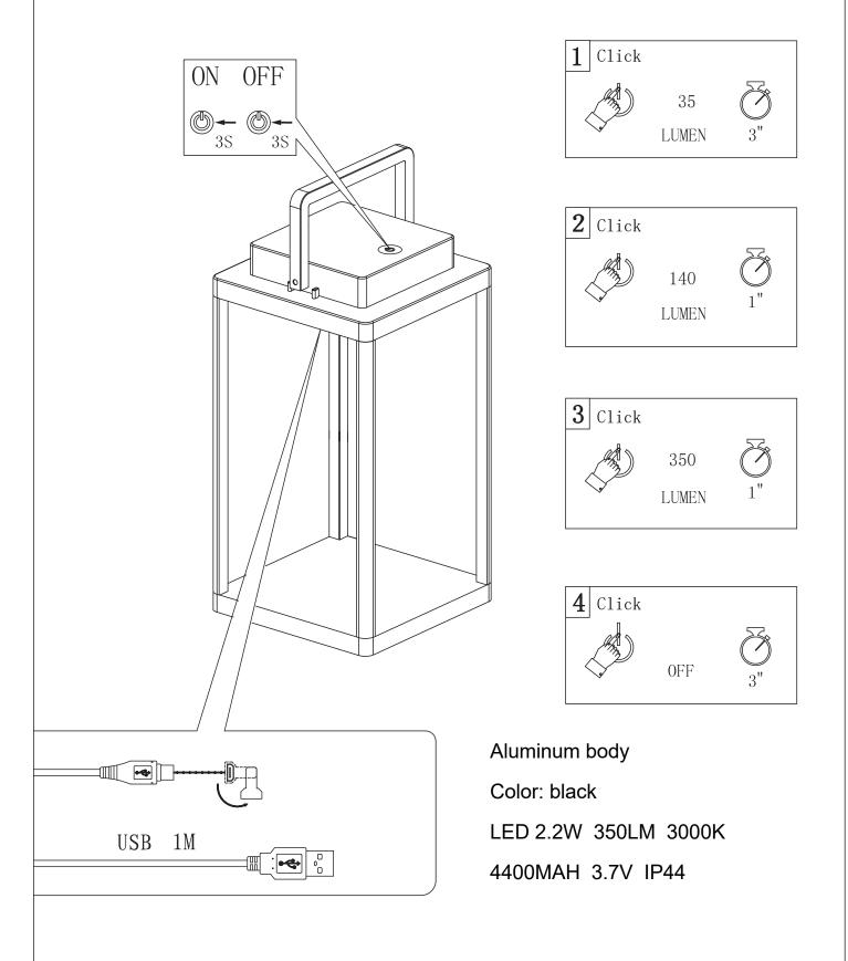
**Warning:** Charge your new LED lamp with 5V output and do not exceed the 5 volt. Do not connect with supercharger which shows output of more than 7V, 9V, 12V etc.
