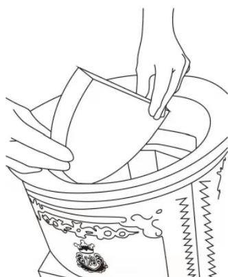
3. Remove the deflector in steel and the parts on the side (F), the front smoke shelf (E) and finally the rear smoke shelf (D).
