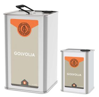
FLOOR OIL is linseed oil from which the nondrying ingredients have been removed with our unique refining method. It penetrates the substrate and dries quickly through a reaction with the oxygen in the air to linoxyn, a natural polymer with excellent adhesion. It is non-biodegradable, waterrepellent and resistant to fats, petroleum products, salts and household acids.
