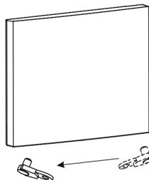
8. Fit the appliance door onto the bearing pin of the bottom door hinge and press it gently against the appliance.
