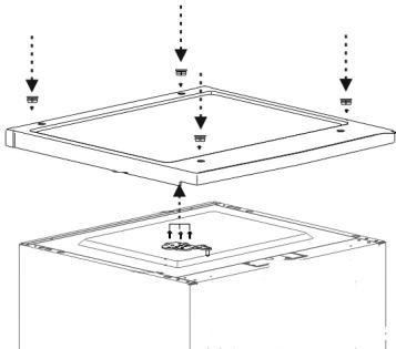
12. Replace the lid of the appliance, screw it tight and replace the screw covers.
