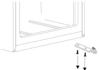
5. Loosen the nut securing the pin to the bottom door hinge and fit the pin with a washer into the other hole. Fix the pin with the nut.
