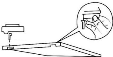
3. Tilt the appliance slightly backwards and unscrew the front adjustable feet from the appliance.
