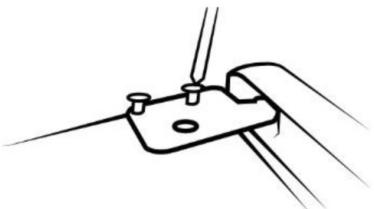
4. Loosen the screws holding the bottom door hinge and remove the door hinge.
