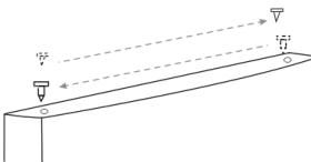
10. Align the door. Insert the top door hinge with the bearing pin into the bushing on the top of the door and tighten it firmly.
