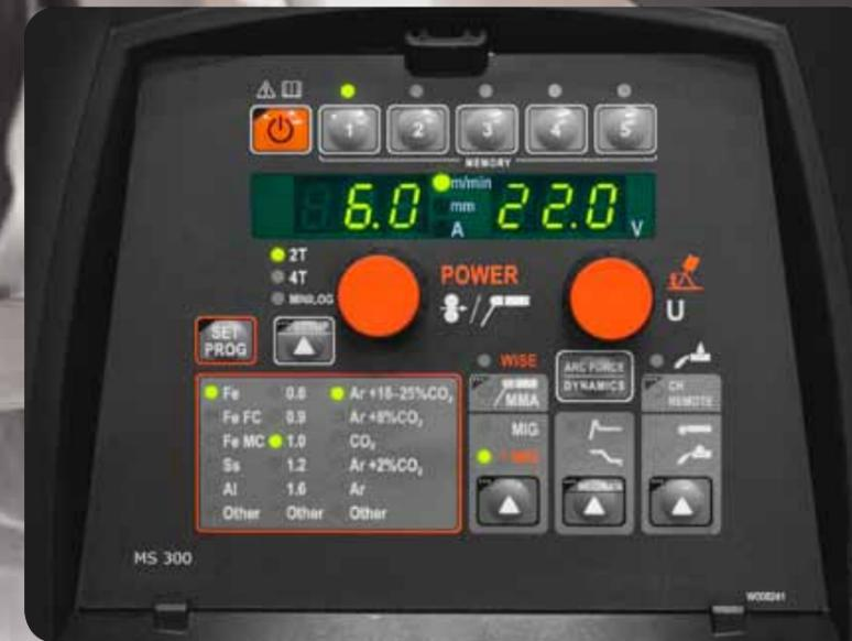
**Synergic FastMig M packages** contain an MS control panel, which includes easy-to-use synergic functionality and a rich selection of additional features for optimising your welding work. These packages are suitable for professional use in more demanding industrial applications.
